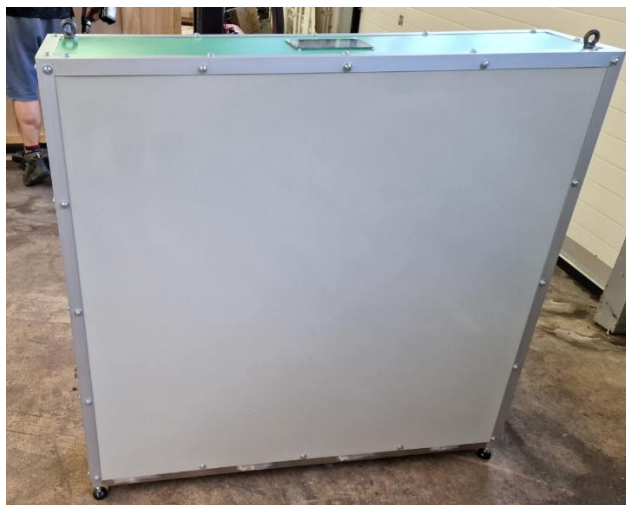
Figure 43 The 10.4kWh proof-of-concept battery
