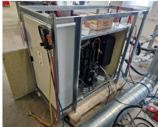
Figure 7 Control Cabinet and refrigeration cycle of R290 35kW BW-HP on test bench
