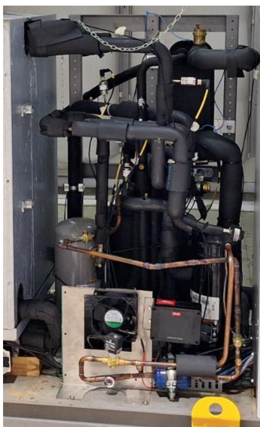
Figure 21 : Refrigerant circuit main components without enclosure
