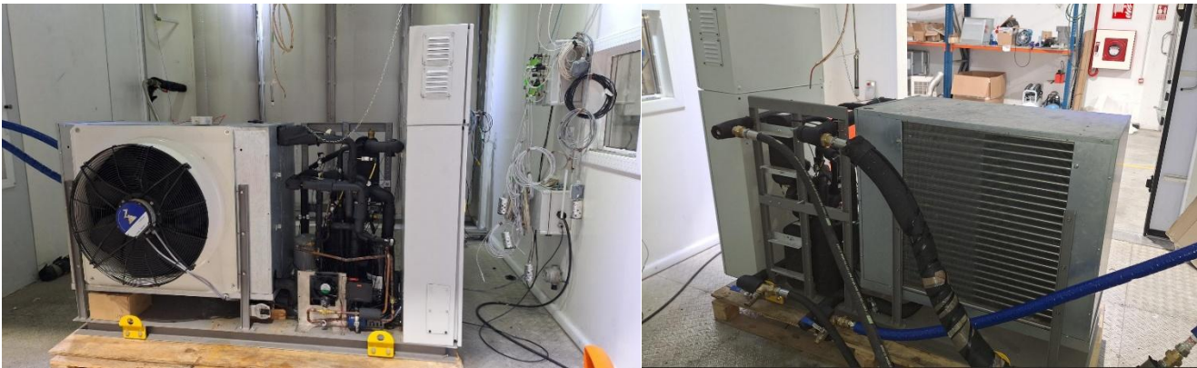
Figure 30 DSHP installed in the climatic chamber to verify the carried-out adaptations
