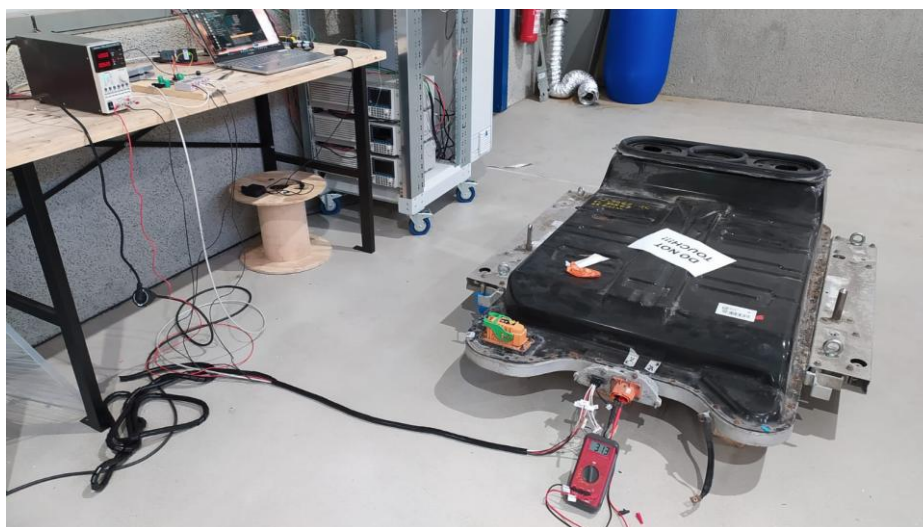
Figure 51 Renault ZOE Gen1 22kWh unlocking setup
